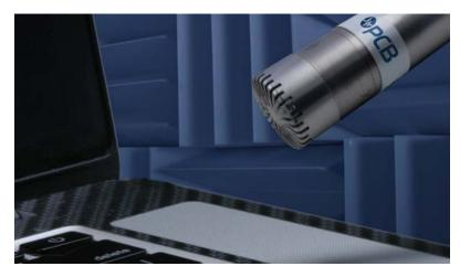
Easily make measurements to 6 dB A-weighted using the Model 831 sound level meter paired with the 378A04 low noise microphone and preamplifier. Due to the innovative design of the 378A04 which uses a prepolarized microphone and ICP (constant current) interface, the combination produces a highly portable system that is battery powered and intuitive to use.
